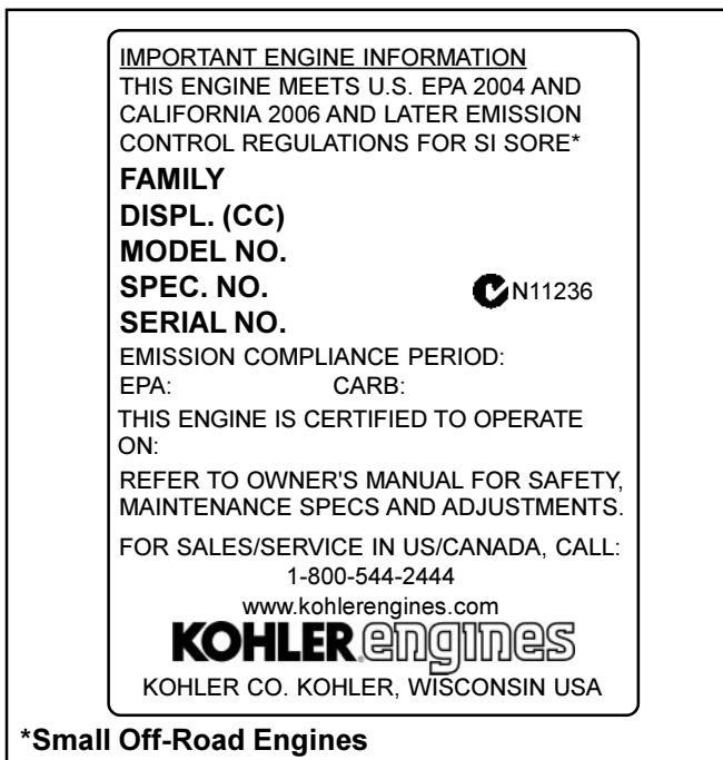
Figure 4. Engine Identification Label.
