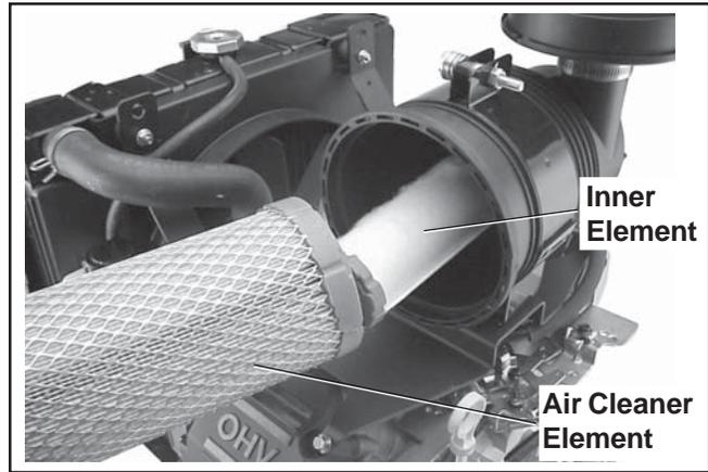
**Figure 14. Air Cleaner Element and Inner Element.**
