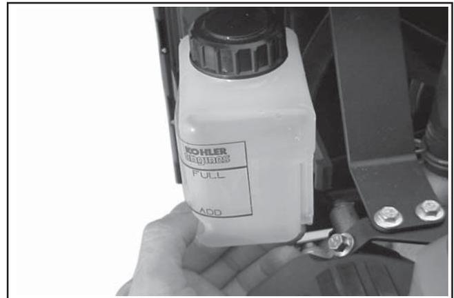
**Figure 13. Removing Reservoir.**
