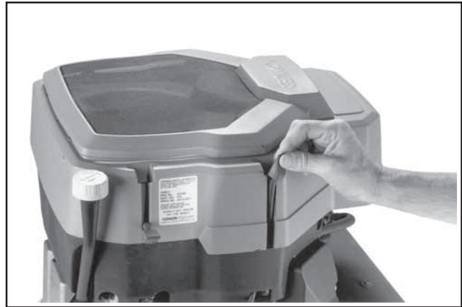
Figure 8. Unhooking Retaining Straps.
