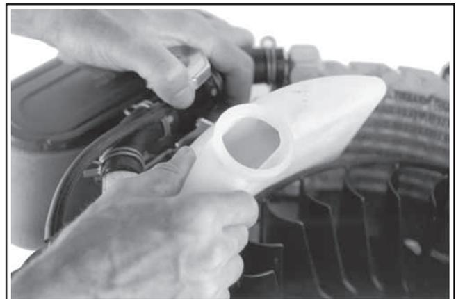
Figure 15. Removing Reservoir.
