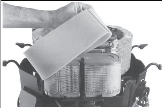
**Figure 17. Removing Precleaner from Paper Element.**
